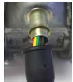
3. Slide the tube and body grommet over the wires. The tube ends should fit inside the ends of the boot and grommet for a sealed finish.
