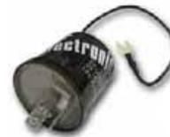
If you decide to use a stock bi-metal flasher, we recommend a standard-duty flasher instead of a heavy-duty flasher. If your turn signal circuit includes front and rear LED turn signals, the circuit will not have enough resistance load to operate a heavy-duty bi-metal flasher, so the no-load flasher will be required for both the turn signal and emergency flashers.
