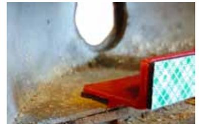
3. Attach the larger angle brackets centered into the main light pocket. There is a small lip on the bracket that sits against the taillight housing lip.
