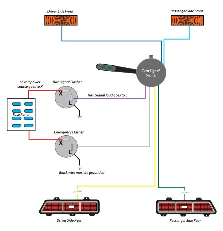
Refer to the DIGI-TAILS wiring schematic for wiring the DIGI-TAILS LED panels.
